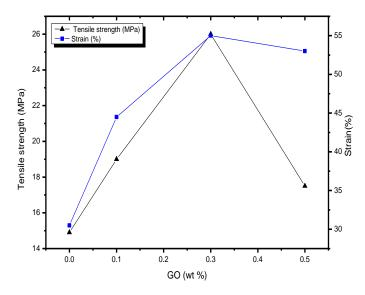
Figure6- Tensile strength (a) and tensile strain (b) of composite hydrogels having different graphene oxide nanosheet (GONS) content [69] (Modified).
