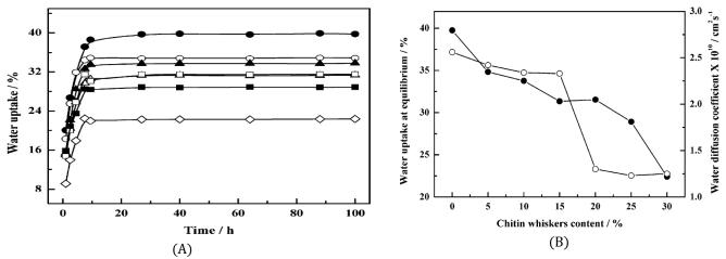
Figure 7: Water uptake at equilibrium of glycerol soy protein isolate sheet (•) and SPI/CHW composites of SPI-5(0), SPI-10 (♠), SPI-15 (Δ), SPI-20 (□), SPI-25 (•) and SPI-30 (◊) composite conditioned at 98 RH% as a function of time (A) and water uptake at equilibrium (•) and water diffusion coefficient (o) as a function of chitin whiskers content for composites conditioned at 98 % RH(B) [15].
