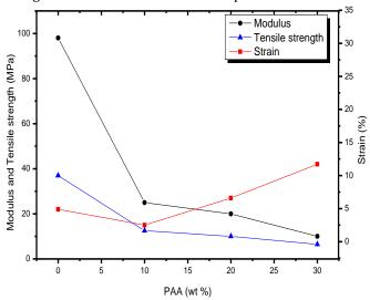
Figure 5- Mechanical properties of gelatine gel reinforced PAA. [68] (Modified).
