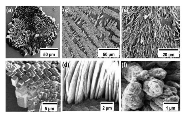
Figure 11 SEM images of the development of the planar films into microarrays by the subsequent overgrowth without any additives for visual determination of the polymorphs: (a, b) calcite; (c, d) vaterite; (e, f) aragonite [80].
