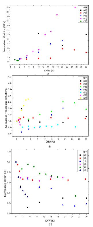
Figure 4- Normalised (against matrix) properties of CHW reinforced composites at different percentage laoding of CHW (A) Modulus, (B) tensile strength and (C) strain at hreak
