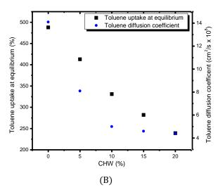
Figure 8: - Variation in toluene uptake of PNRev (•), PCH5ev (o) PCH10ev (△), PCH15ev (Δ), and PCH20ev (□) samples as a function of time at room temperature (25 °C)(A) and toluene uptake at equilibrium and toluene diffusion coefficients in CHW/Vulcanized NR Composites immersed in toluene (B). [47]
