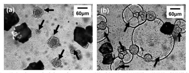
Figure 12 - Optical micrographs of calcium carbonate grown at  $10 \,^{\circ}$ C with  $2.4 \, x 10^{-3} \,$ wt % PAA250k on  $100 \,^{\circ}$ C (a) and  $260 \,^{\circ}$ C baked (b) chitosan. Arrows indicate planar films. Black shadows are granular particles [80].
