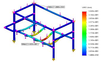
*Figure 5: Distribution of the resultant displacement of the machine frame members*
