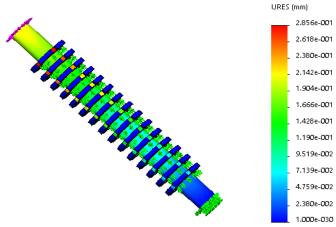
*Figure 10: FE model of the resultant linear displacement variation due to torsion*
