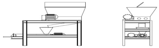
Figure 2: Orthographic view of the plastic recycling machine
