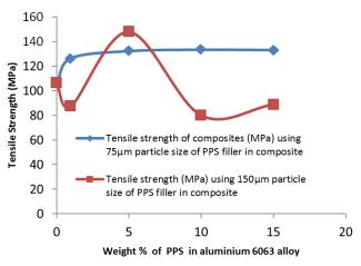
Figure 10: Tensile strengths of AA6063 alloy and PPS-AIMMCs
