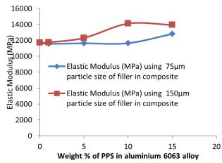
Figure 11: Elastic moduli of AA6063 alloy and PPS-AlMMCs
