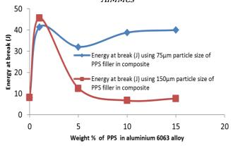
Figure 13: Energies at break of AA6063 alloy and PPS-AIMMCs
