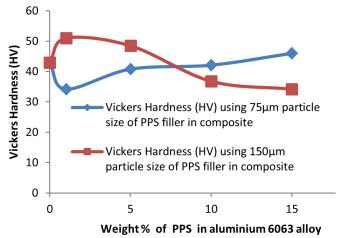
Figure 14: Vickers hardness of AA6063 and PPS-AIMMC composites
