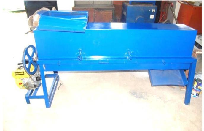
Figure 4 Picture of the Side View of Type 2 Cassava Peeler
