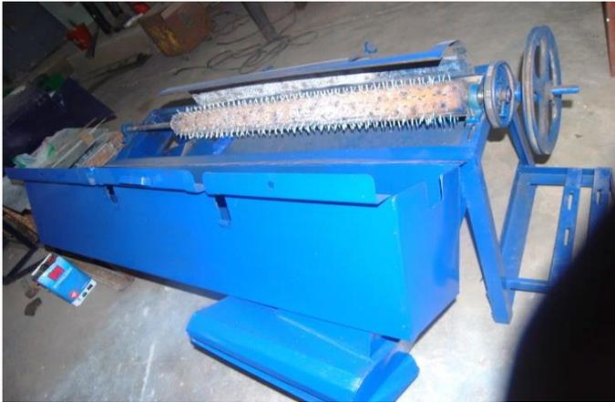
Figure 3 Internal Component of Type 2 Cassava Peeling Machine
