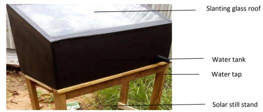
Figure 2: Isometric view of the slanting-type solar water distillation (SSWD) kit
