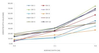
*Figure 1: Variation of corrected N-values with boring depth*
