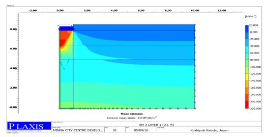
*Figure 7: Numerical analysis result of stress distribution up to the collapse of the soil body at 0.6 m embedment depth (BH 3)*
