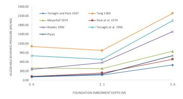
*Figure 2: Variation of allowable bearing pressure with foundation embedment depth (BH 3)*
