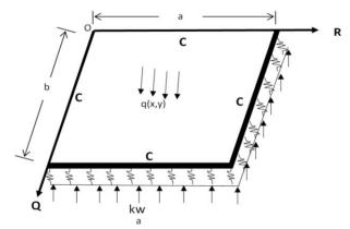
Figure 1: An all clamped rectangular thin plate on elastic foundation
