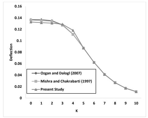
Fig. 2 Variation of the non dimensional central deflection with K for clamped supported plate subject to concentrated load
