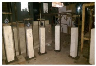
*Plate 1: Laboratory setup for measuring shrinkage strain in the specimens*
