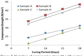
*Figure 3: Variation of compressive strength with curing period of the four samples of concrete*
