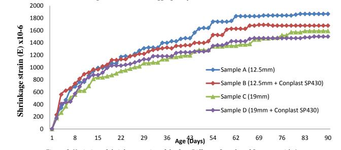
Figure 2: Variation of shrinkage strains of the four Different Samples of Concrete with Age.
