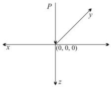
Figure 1: Point load P acting at the origin of a semi-infinite (half space) soil.
