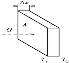
*Figure 4. Conduction of heat transfer process through surfaces with different temperature, Source: Modi et al. [21].*
