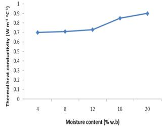
*Figure 6. Variation of thermal heat conductivity with moisture content of Prosopis africana seeds (Okpeye)*
