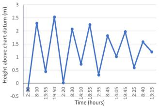
*Figure 2: Predicted tides above chart datum for Lagos Harbour for June 1, 2017 at five minutes Interval from 0:00 hour*
