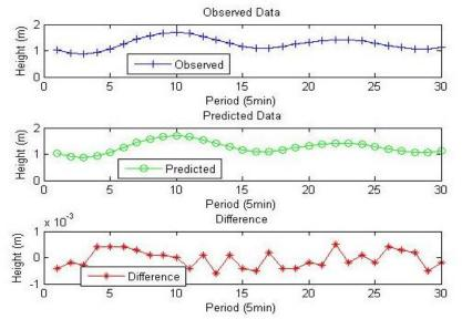
Figure 4: Sample of hourly observed and predicted tidal data above chart datum
