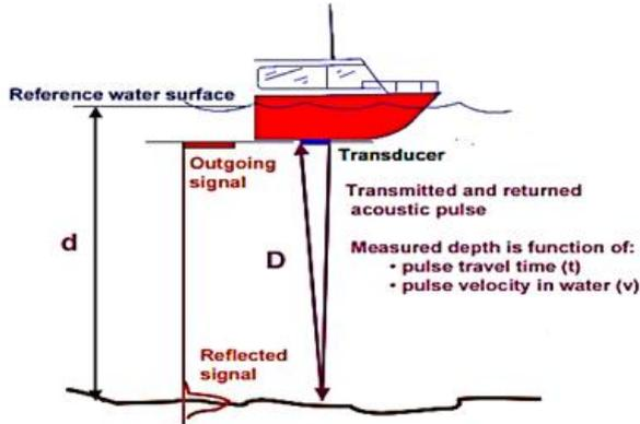
Figure 1: Principle of acoustic depth measurement.
