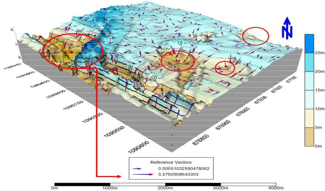
Figure 5: The magnitude and direction of flow of Kainji reservoir
