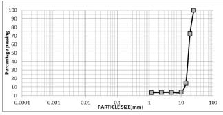
*Figure 2: Particle Size Distribution Curve for Coarse Aggregate*
