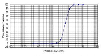
Figure 1: Particle Size Distribution Curve for Sand
