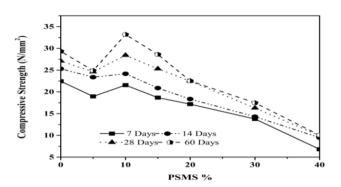
Figure 3: Variation of Compressive Strength with Percentage PSMS and Age
