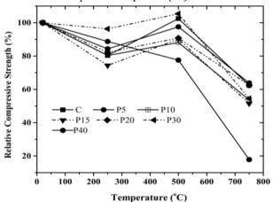
*Figure 5: Relative strength of the concrete specimens subjected to elevated temperatures.*
