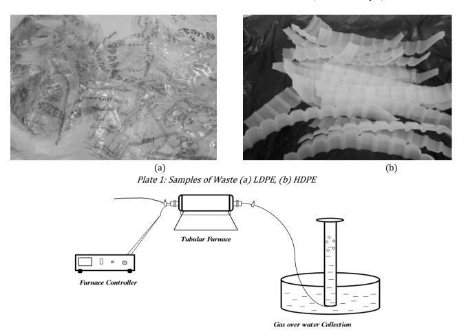
Figure 1: Schematic Drawing of Pyrolysis Apparatus (Effect of Heating Rate)
