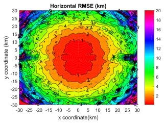
*Figure 6: Horizontal PE RMSE for the directional rotating antenna multiangulation system with AOA estimation error of 2*<sup>0</sup>
