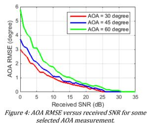
The AOA RMSE at SNR of 15 dB for AOA of 30<sup>0</sup>, 45<sup>0</sup> and 60<sup>0</sup> are 0.59<sup>0</sup>, 0.75<sup>0</sup> and 1.10<sup>0</sup> respectively. This means that at the same SNR value, the AOA RMSE for 30<sup>0</sup>, 45<sup>0</sup> and 60<sup>0</sup> are different. Thus, the AOA RMSE of the beamforming AOA estimation depends on the AOA and the received SNR. Due to the geometrical configuration of the GRSs, the AOA of the signal transmitted by an
