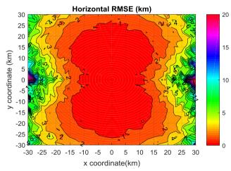
Figure 5: Horizontal PE RMSE for the developed multiangulation system with beamforming Bartlett's AOA estimation method.
