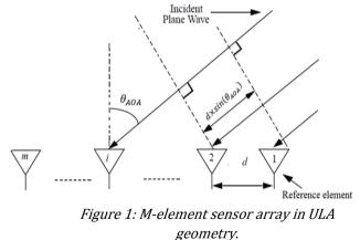
Given an *m*-element sensor array in a ULA geometry as shown in Figure 1, a radiated narrow band signal defined in Eq. (1) from a source impinges on the sensor array with an angle of arrival,  $\theta_{AOA}$ .
