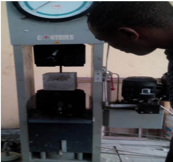
Fig. 4 Experimental set-up of the pull out test
