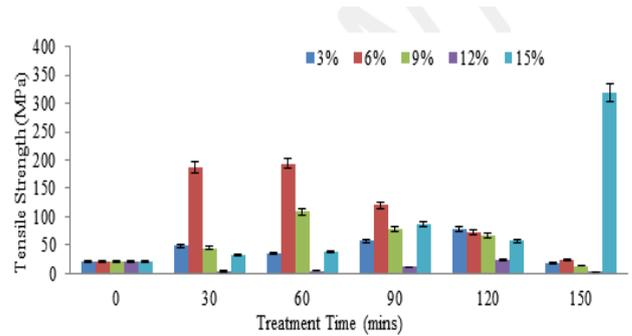
Figure 3: Tensile strength of AC treated *C. populnea* fibers
