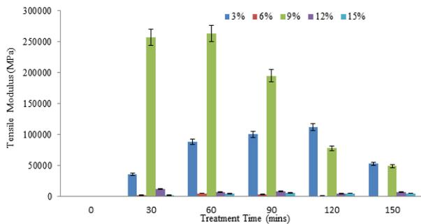
Figure 4: Tensile modulus of AC treated *C. populnea* fibers
