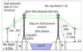
Figure 3: Side view of designed 33kV overhead line
