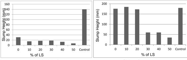
a) 0.6 w/c b) 0.7 w/c Figure 1: Effect of Replacement on Workability (1:1.5:3 mix)
