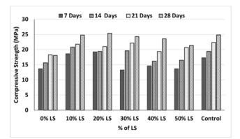
*Figure 3: Variation of Compressive Strength with Age at Different % of LS (1:2:4 mix and 0.6 w/c)*
