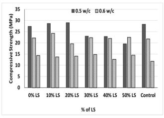
*Figure 4: Variation of 28<sup>th</sup> Day Compressive Strength with Water/Cement Ratio at Different % of LS (1:1.5:3 mix)*
