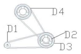
Figure 1: Belt Pulley Double Reduction Mechanism
