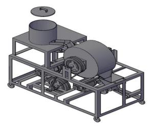
Figure 2: Solid Model Isometric View of the Improved Plant Processing Machine
