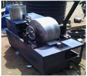
Figure 3: Fabricated Improved Plantain Processing Machine
