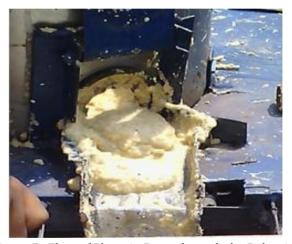
Figure 5: Flow of Plantain Paste through the Pulverizer
