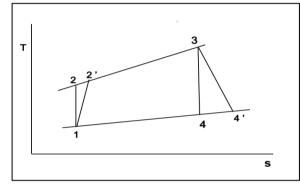
Figure 1: The T-s diagram of a Gas Power Plant
