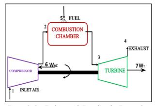
*Figure 2: Gas Turbine with Encoding for Exergy Cost Analysis*
