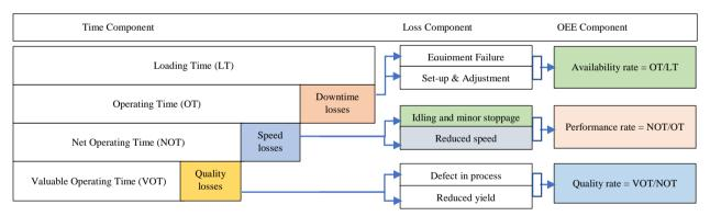
Fig.1 The OEE fundamental components according to Nakajima (After [7] in [6])
