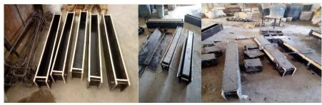
Figure 3: Wooden Formwork, Cast Beams and Cubes
