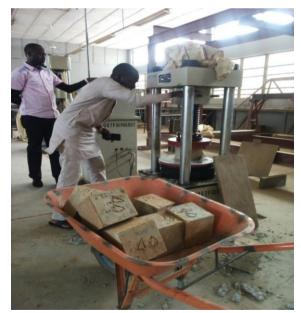
*Figure 6: Compressive Strength Tests on Cubes at 28 Days*
