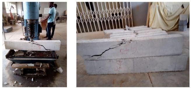
Figure 7: Beam Test Set Up and Tested Beams
