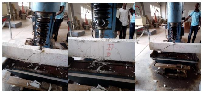
Figure 8: Shear Failures in Beam Test
