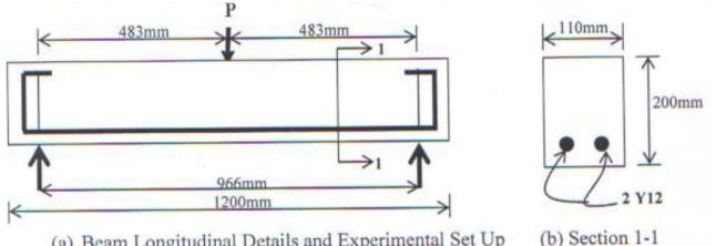
(a) Beam Longitudinal Details and Experimental Set Up Fig 4: Beam Details and Test Setup
