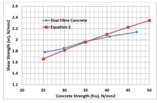
Fig 11: Comparison of Equation (2) and the Shear Strength of Sisal Fibre Reinforced Concrete
