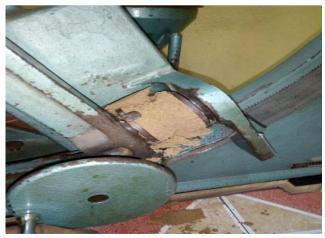
Figure 3: Green Compression Testing using Ridsdale Sand Compression Tester
