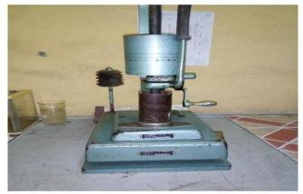
Figure 2: Ramming of Sand/Binder Formulations using Ridsdale Rammer
