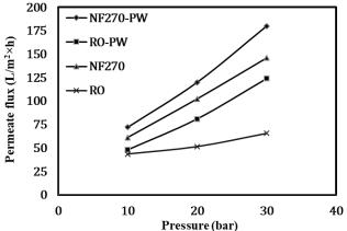
Figure 2: Pure water (PW) flux and permeate flux as function of feed pressure for the NF and RO membranes at (22±2) <sup>o</sup>C.
