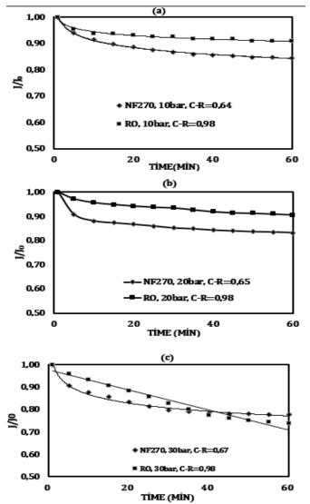
Figure 4: Relative flux decline compared to initial permeate flux for different experimental conditions at ambient temperature (22±2) <sup>o</sup>C. Codes: NF270nanofiltration, RO-reverse osmosis membrane, Coriginal mine water, R-rejection.
