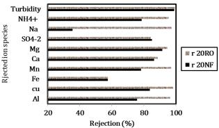
Figure 3: Selectivity of the NF and RO membranes at ambient temperature  $(22 \pm 2)$ <sup>0</sup>C and TMP of 20 bar.
