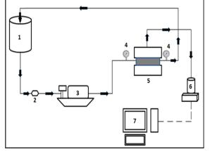
Figure 1: Flow diagram of laboratory scale membrane systems (1. Waste water tank 2. Flow meter 3. High pressure pump 4. Pressure gauge 5. Membrane housing 6. Electronic balance 7. Computer).
