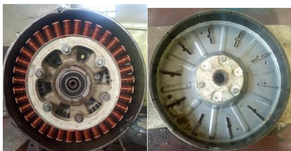
*Figure 8: Developed Stator and Rotor Compartments*
