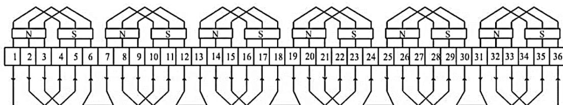
Figure 3: SPSMPMSG Winding Diagram
