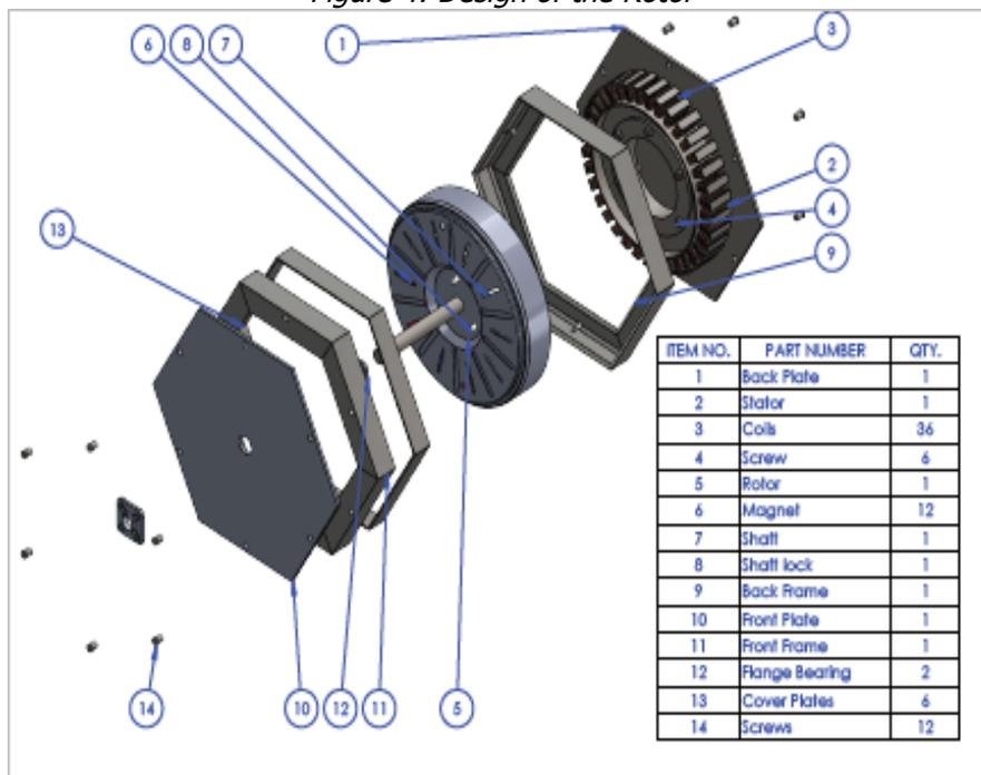
Figure 5; Complete Assemblage of the SPSMPMSG
