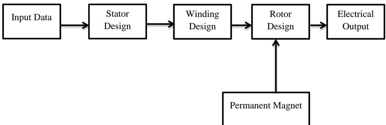
Figure1: Design Sequence for Permanent Magnet Generator
