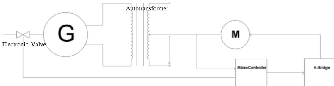
Figure 6: Voltage regulator for the Generator
