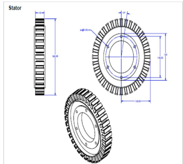
Figure 2: Design of the Stator
