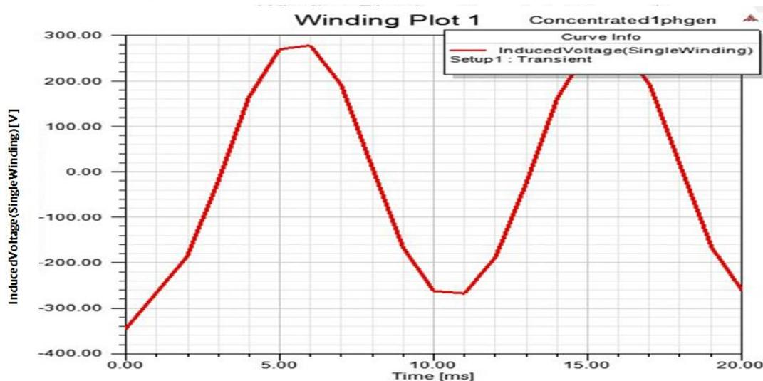
*Figure 7: Output Voltage Waveform of the Generator*
