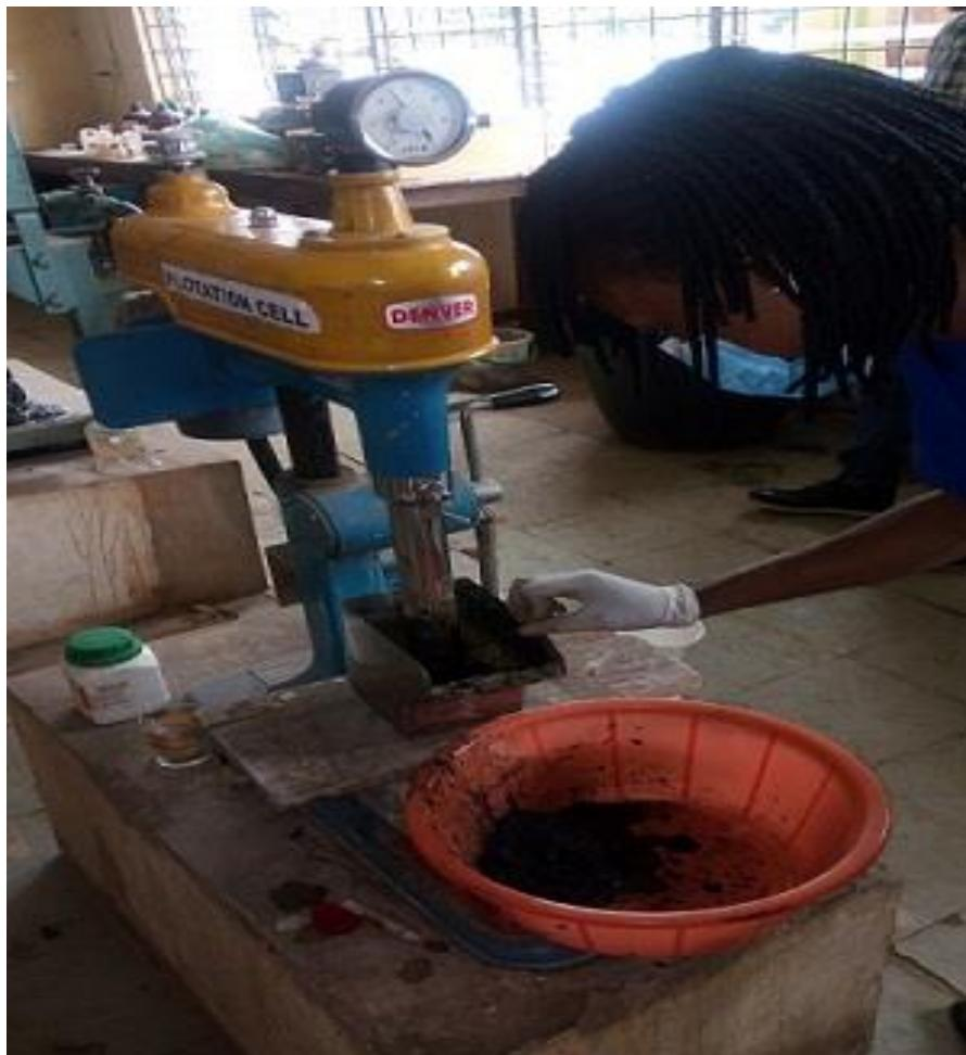
Plate 1: Denver Flotation Cell
