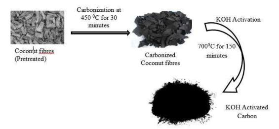
Figure 2: Diagram showing the production process of activated carbon from coconut fibres.
