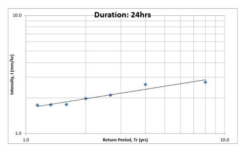
Figure 9: Intensity-Return Period Curves of Abuja for Duration of 24hrs
