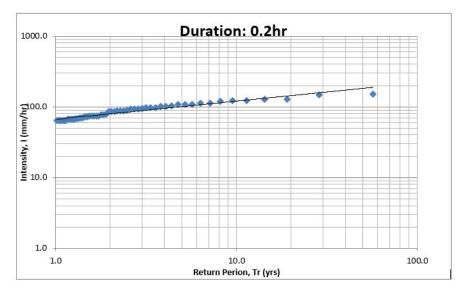
Figure 1: Intensity-Return Period Curves of Abuja for Duration of 0.2hr
