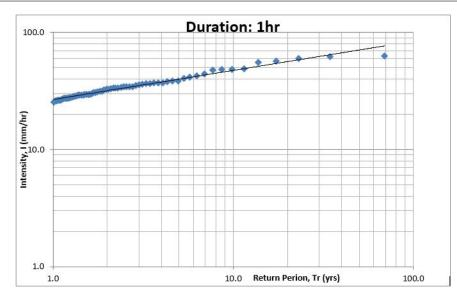
Figure 4: Intensity-Return Period Curves of Abuja for Duration of 1hr
