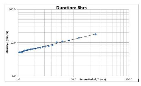
Figure 7: Intensity-Return Period Curves of Abuja for Duration of 6hrs
