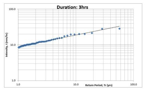
Figure 6: Intensity-Return Period Curves of Abuja for Duration of 3hrs
