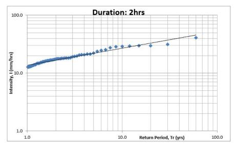
Figure 5: Intensity-Return Period Curves of Abuja for Duration of 2hrs
