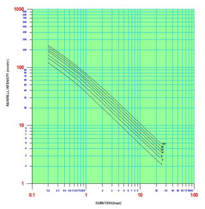
Figure 10: Intensity-Duration-Frequency Curves for Abuja
