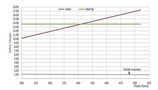
Figure 3 Variation in depth with the Safety Margin of Anogeissus Schimperi Timber Bridge Beam
