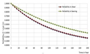
Figure 1: Reliability of Anogeissus schimperi Timber Bridge Beam
