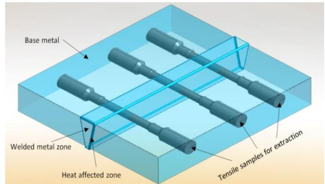
Figure 5: Format for extraction of tensile specimen
