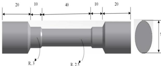
Figure 4: Sample of tensile specimen. (All dimension in, mm.)
