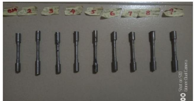
Figure 6: Extracted tensile specimens machined for the Test.
