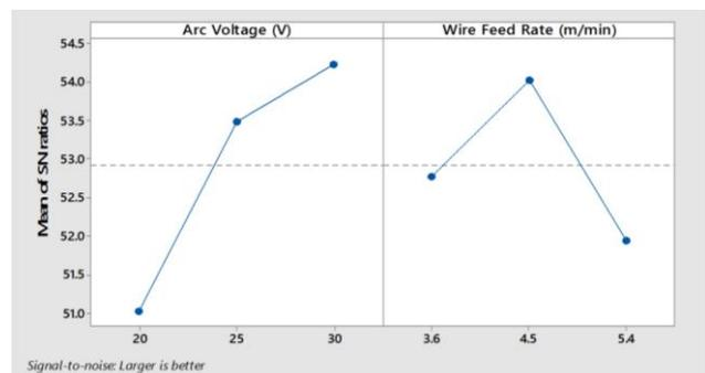
Figure 7: Main effects plot for Tensile strength
