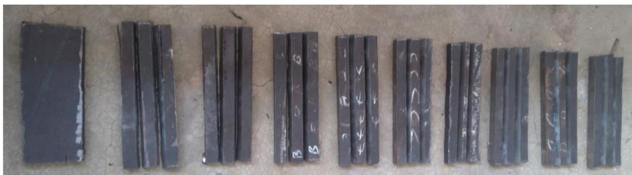
Figure 2: The API X70M base material prepared for welding.
