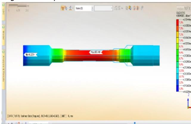
Figure 11: Maximum and minimum solid stresses at break
