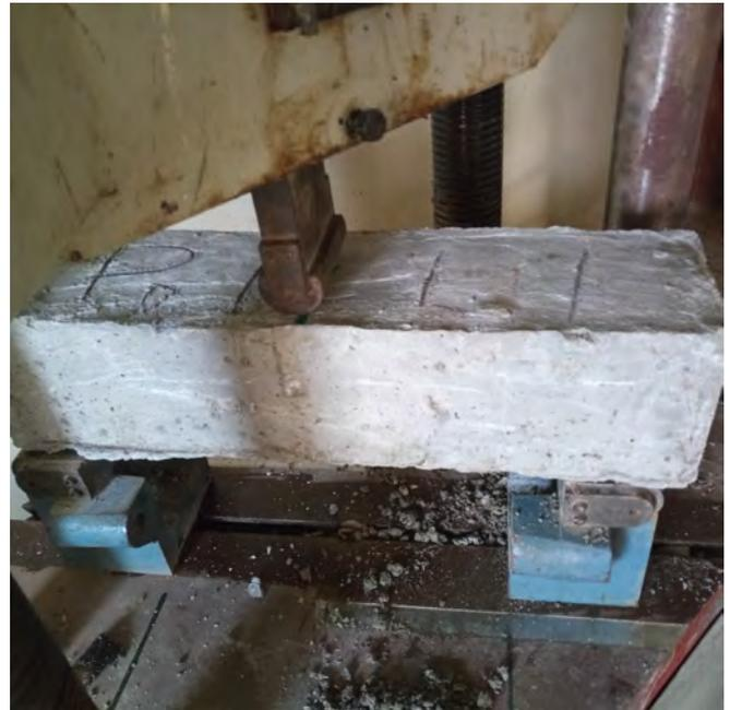
Figure 2: Flexural strength test of reinforced concrete beam not (location map of study areas).
