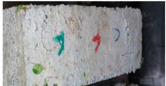
Figure 6: Beam buried in Fresh water after 1 year.
