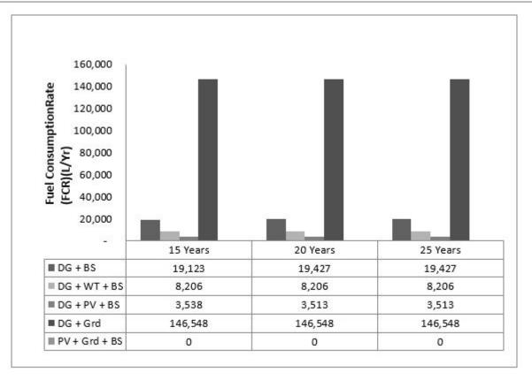
Figure 5: Simulation results for fuel consumption rate.
