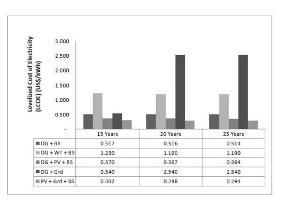
Figure 4: Simulation results for levelized cost of energy.
