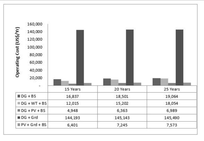
Figure 3: Simulation results for operating cost.
