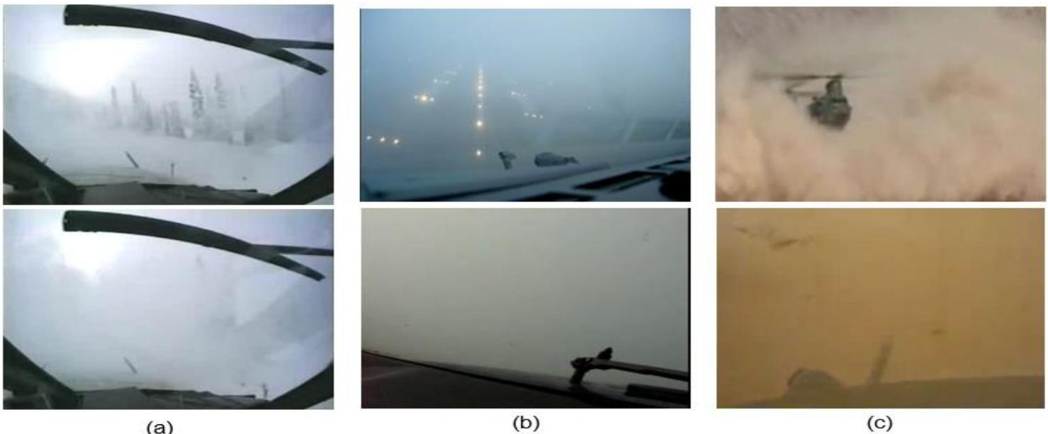
**Figure 1:** Helicopter visibility in poor weather conditions (a) Whiteout due to snow (b) Foggy condition and (c) Brownout condition due to dust [18]
