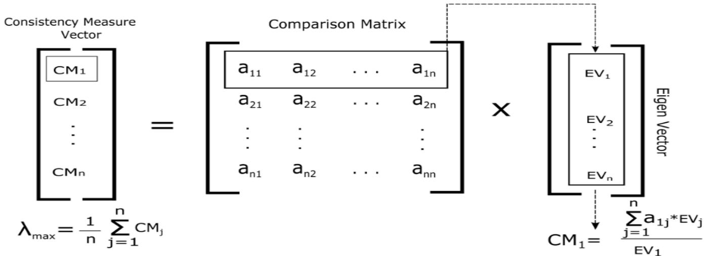
Figure 5: Consistency Measure Calculation [25]
