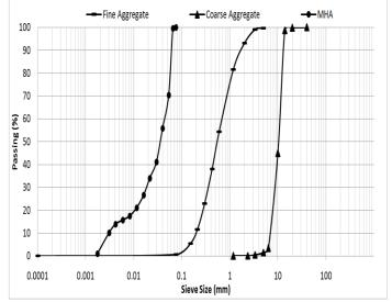
Figure 1: Grading of Aggregates and Millet Husk Ash
