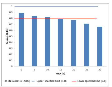
**Figure 3:** Variation of Passing Ability for increasing Millet Husk Ash Content in Self-Compacting Concrete
