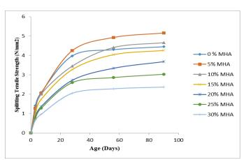
**Figure 13:** Splitting Tensile Strength of Self-Compacting Concrete modified with Millet Husk Ash
