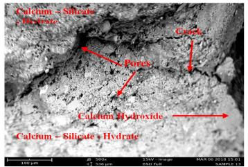
**Figure 9:** Scanning Electron Micrograph of Control Sample (0 % Millet Husk Ash) of Self Compacting Concrete at 90 days Curing Age
