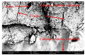
**Figure 8:** Scanning Electron Micrograph of Control Sample (0 % Millet Husk Ash) of Self Compacting Concrete at 28 days Curing Age
