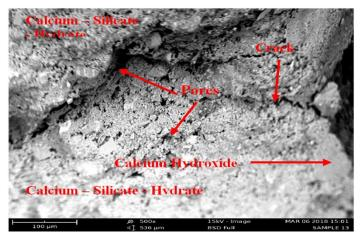
**Figure 11:** Scanning Electron Micrograph of Self Compacting Concrete Specimen containing Optimum Millet Husk Content Sample (5 % Millet Husk Ash) at 28 days Curing Age
