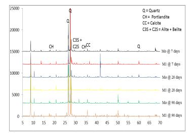
**Figure 6:** XRD Pattern for Self-Compacting Concrete modified with 5 % Millet Husk Ash as Replacement of Cement
