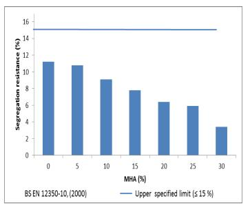
**Figure 4:** Variation of Segregation Resistance for increasing Millet Husk Ash Content in Self-Compacting Concrete
