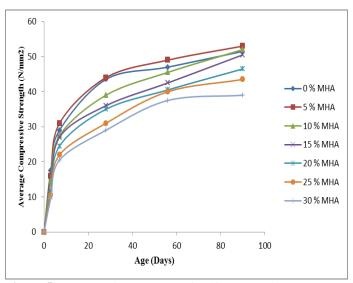
**Figure 5:** Compressive Strength of Self-Compacting Concrete modified with Millet Husk Ash
