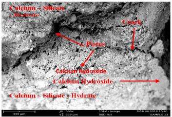
**Figure 12:** Scanning Electron Micrograph of Self Compacting Concrete Specimen containing Optimum Millet Husk Content Sample (5 % Millet Husk Ash) at 90 days Curing Age
