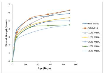
Figure 14: Flexural Strength of Self-Compacting Concrete modified with Millet Husk Ash
