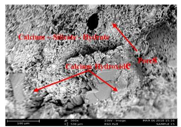
**Figure 7:** Scanning Electron Micrograph of Control Sample (0 % Millet Husk Ash) of Self Compacting Concrete at 7 days Curing Age
