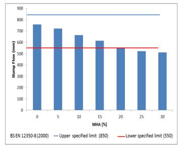
**Figure 2:** Variation of Slump Flow for increasing Millet Husk Ash Content in Self-Compacting Concrete
