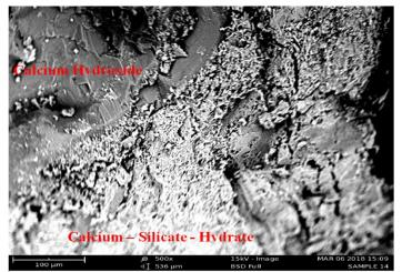
**Figure 10:** Scanning Electron Micrograph of Self Compacting Concrete Specimen containing Optimum Millet Husk Content Sample (5 % Millet Husk Ash) at 7 days Curing Age
