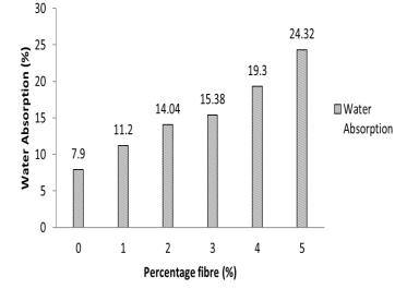
Figure 4: Water absorption of produced block samples
