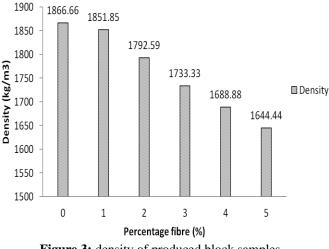
Figure 3: density of produced block samples
