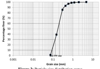
Figure 2: Particle size distribution curve
