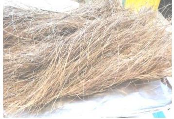
Figure 2: Washed and dried coir fibres
