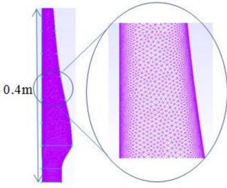
Figure 2: Meshing around the blade
