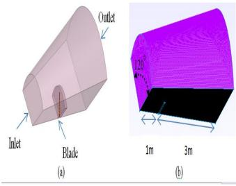
Figure 1: Diagram of the flow domain
