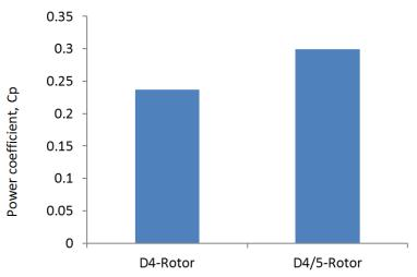
Figure 4: Power coefficient values for the two rotors
