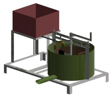
Figure 1: Isometric drawing of manual egusi washing machine
