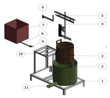
Figure 2: Explored view drawing of manual egusi washing machine
