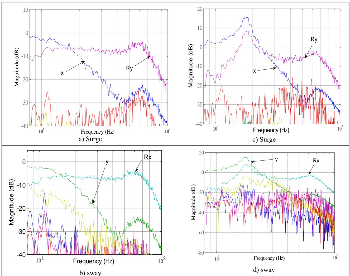
**Figure 1:** Simulation results of cross coupling characteristics for the modal space (right column, a-b) and conventional joint space controller (left column, c-d)
