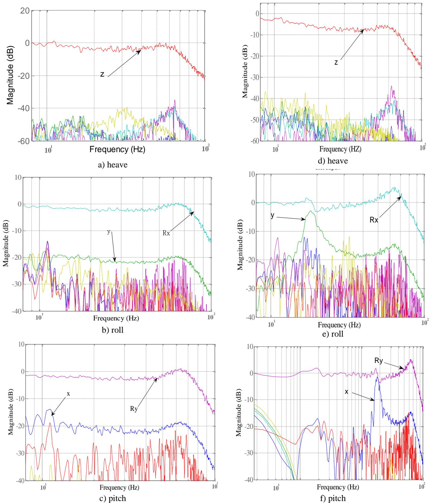
**Figure 2:** Simulation results of cross coupling characteristics for the modal space (right column, a-e) and conventional joint space controller (left column, d-f)
