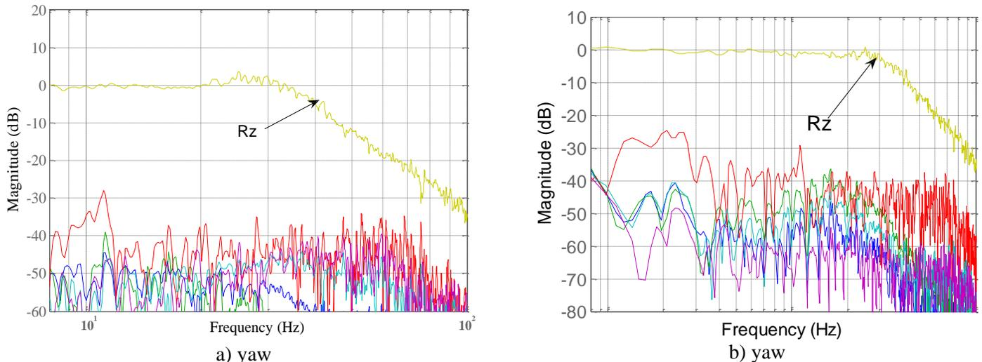
**Figure 3:** Simulation results cross of coupling characteristics for the modal space (right column, a) and conventional joint space controller (left column, b)
