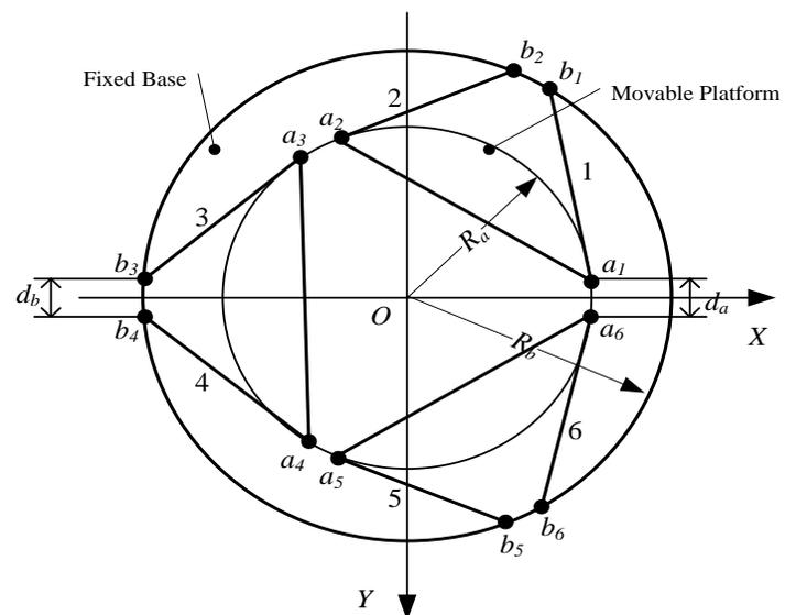
Figure 2: Top view of 6 DOF parallel mechanism
