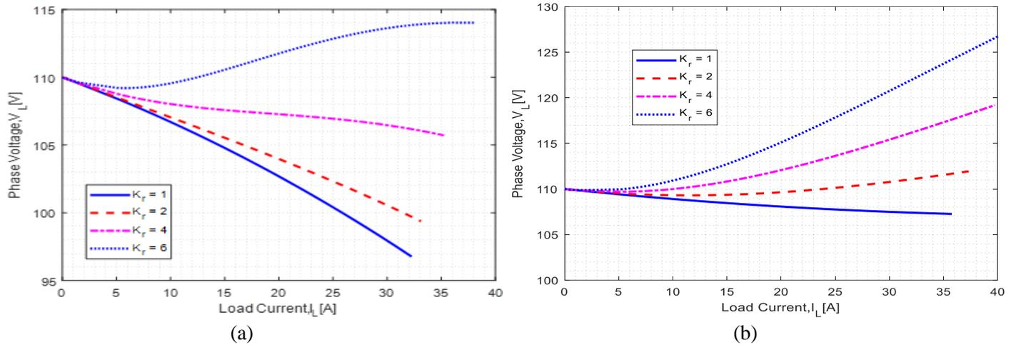
**Figure 4:** Steady-state load characteristic of the IPMSG at different inverse saliency ratios, at rated voltage, nominal speed of 1500 rpm and unity power factor (a) without capacitor (b) with capacitor
