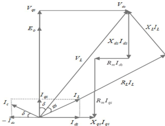
**Figure 3:** The phasor diagram of the IPMSG at lagging power factor
