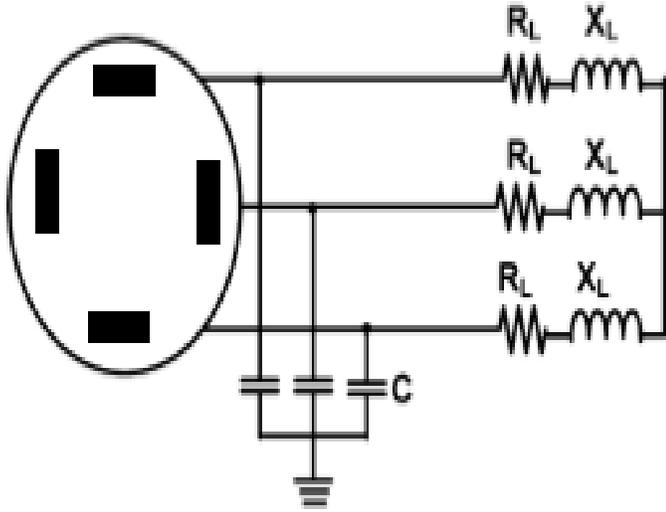
**Figure 1:** Conceptual connection diagram of the three-phase IPMSG [27]
