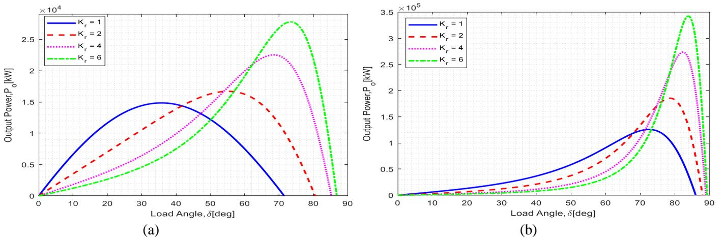
**Figure 5:** Effect of inverse saliency ratio on power-load angle characteristics of IPMSG operating at 1500 rpm and 1.0 power factor (a) without capacitor (b) with capacitor
