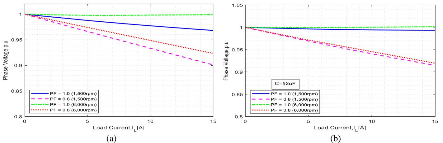
**Figure 6:** Steady-state load characteristic of the IPMSG at different power factors and rotor speed, (a) without capacitor, (b) with capacitor
