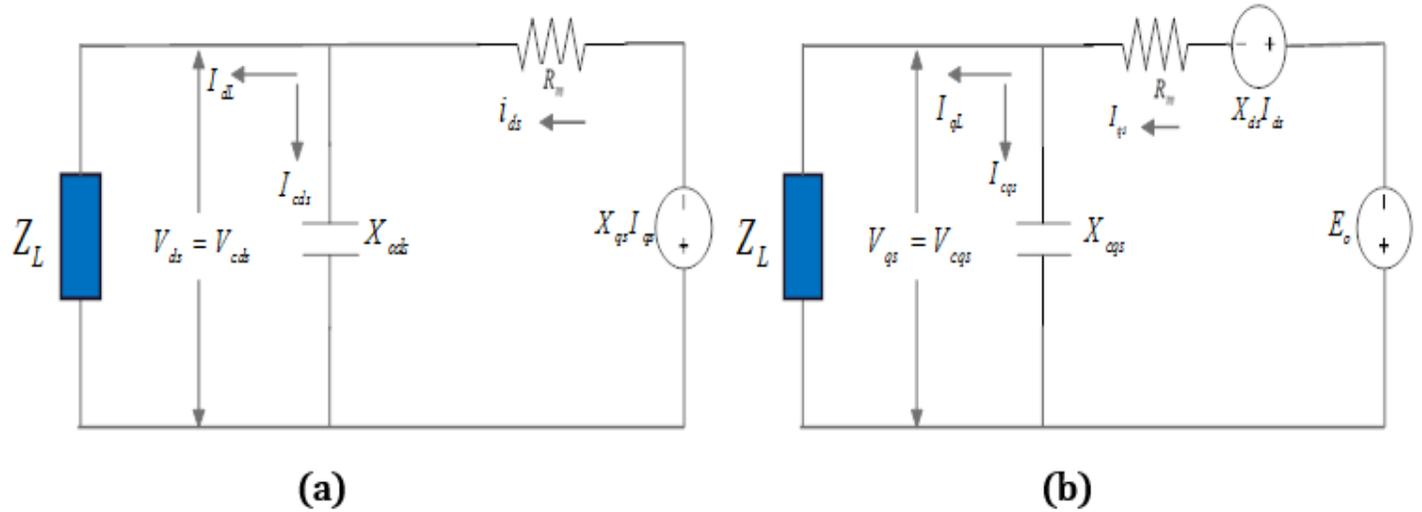
**Figure 2:** The steady-state equivalent circuit of the IPMSG (a) d-axis (b) q-axis
