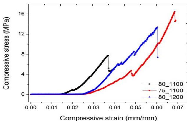
**Figure 5:** Compressive stress as a function of compressive strain for the porcelain samples
