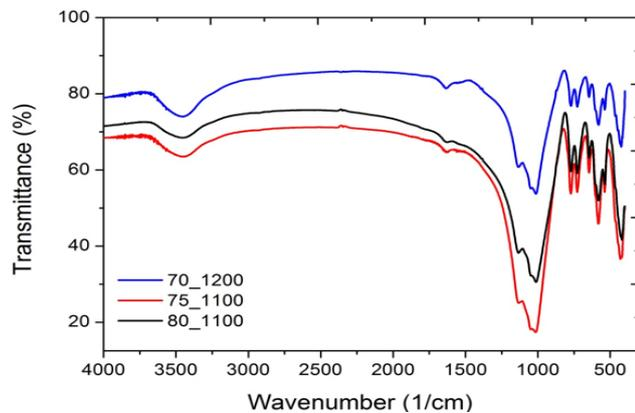
**Figure 4:** Fourier Transform Infra-red plots of 70-1200, 75-1100 and 80-1100 porcelain samples showing the percentage transmittance as a function of the wavenumber
