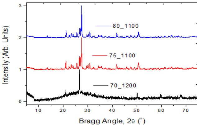
**Figure 2:** X-ray diffraction patterns of samples 70-1200, 75-1100 and 80-1100. The first two digits indicate the amount of feldspar in the porcelain while the last four digits indicate the sintering temperature.
