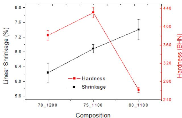
**Figure 1:** A graph of linear shrinkage and Brinell Hardness (BHN) as a function of sample composition at room temperature.
