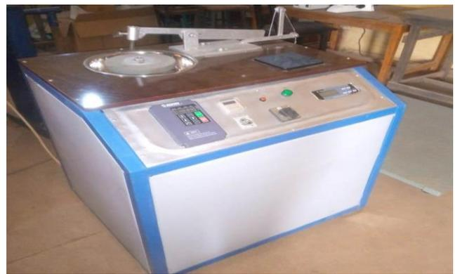
**Figure 1:** Pin-on-Disc wear test machine (Manufactured in Auchu Polytechnic)
