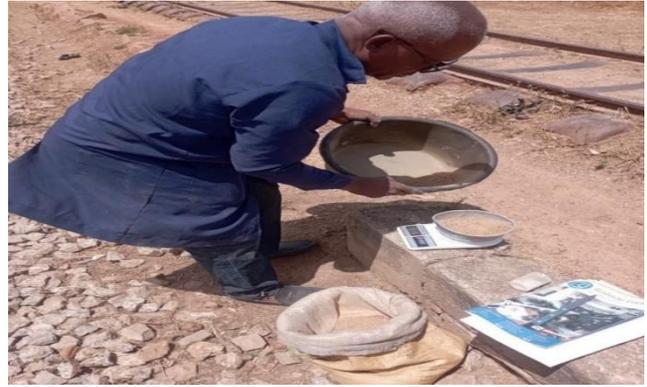
**Figure 8:** Weighing infiltrated fouling materials
