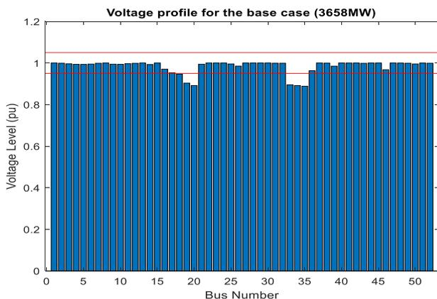
Figure 6: Voltage profile for case one
