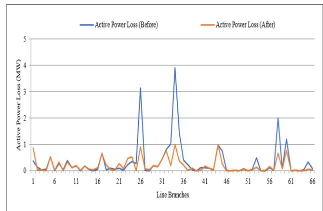
Figure 7: Active power losses before and after integration of PMS-WTGs to the grid
