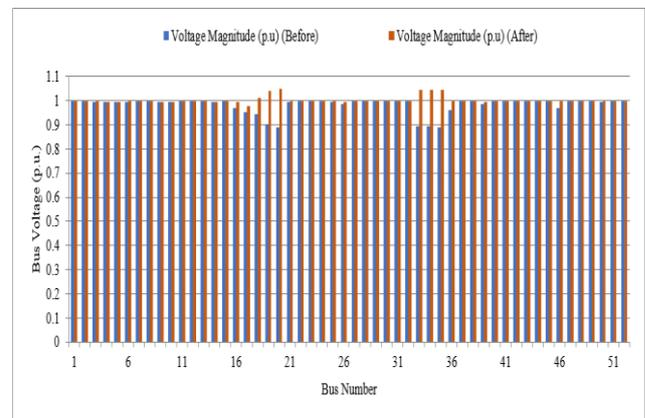
Figure 8: Voltage fluctuations before and after wind integration and ACO
