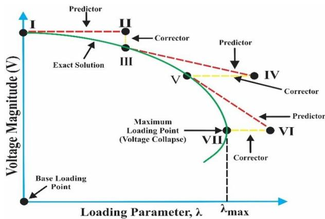
Figure 3: Continuation power flow process [19]
