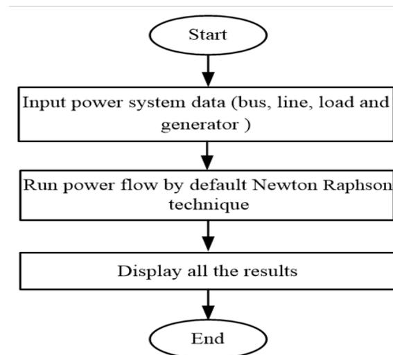
Figure 2: Matpower running process flowchart
