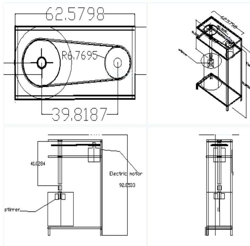
Figure 1: Assembly and isometric drawing of the mixer.
