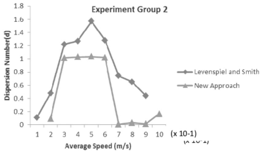
Figure 3: Variation of Dispersion Number with Average Speed for Experiment 2.
