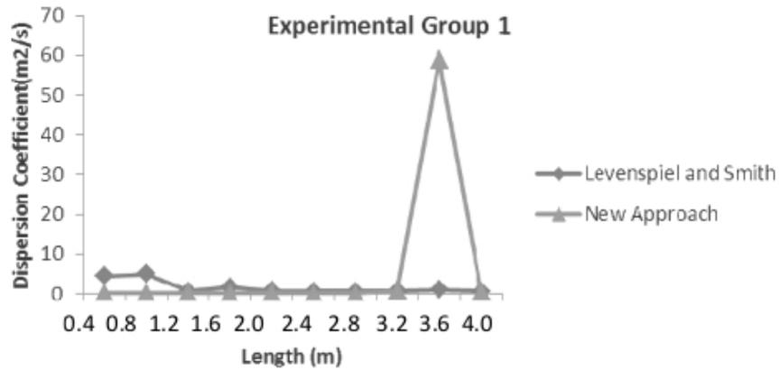
Figure 2: Variation of Dispersion Coefficient with Sampling Length for Experiment 1.
