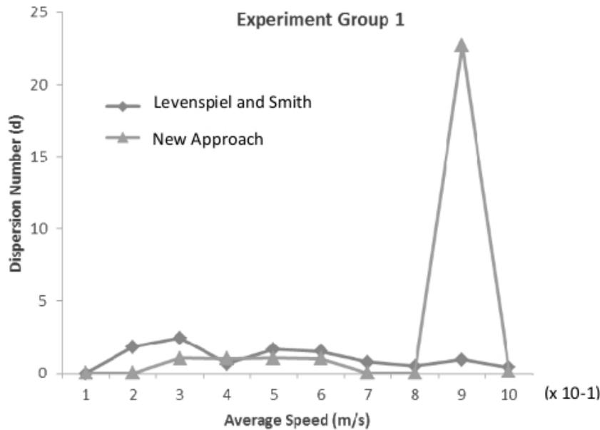
Figure 1: Variation of Dispersion Number with Average Speed for Experiment 1.
