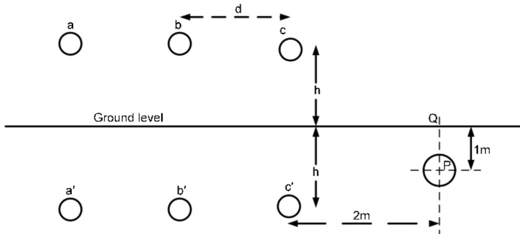
Figure 1: 33-kV line conductors and their mirror images.
