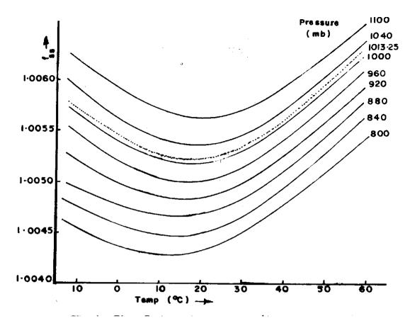
Fig. 4 .the factor  $f_{\rm ss}$  as function of P and T
