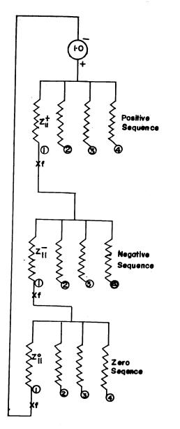
Fig. Al. Intersequence connection for S-L-G Fault.
